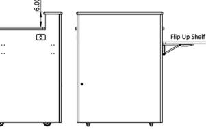
Model **PD3009** podium features a smaller footprint yet retains full size features with a divided interior configured with EIA compliant 14U rack rails on the left side and tower PC storage space on the right.
